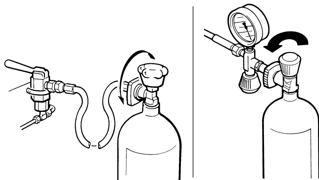
Fig. 9 Connecting air bottle
